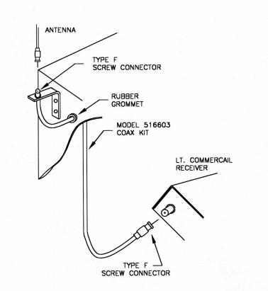
It is recommended that the cable be protected by a rubber grommet, at the point where it passes through the structure.
