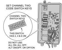
STEP 3 Transmitter code setting. Locate the coding switch on the transmitter and set the eight keys identical to those on the desired channel of the receiver. Be sure they match exactly. If using a two or four-channel transmitter, refer to the coding instructions included with the transmitter for proper system coding.
