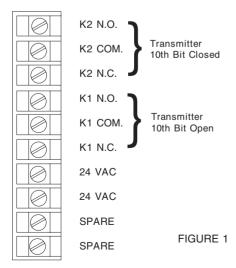
Back the screws on the terminal block off slightly and insert your wiring lugs (or wire) under the appropriate set screw.
